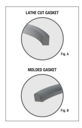
NOTE: This guide is intended only to assist installers with the key differences between installation of a typical spin-on oil filter with a lathe cut gasket vs. less common spin-on oil filters featuring molded gaskets. Follow manufacturer's instructions for the complete oil change procedure.
